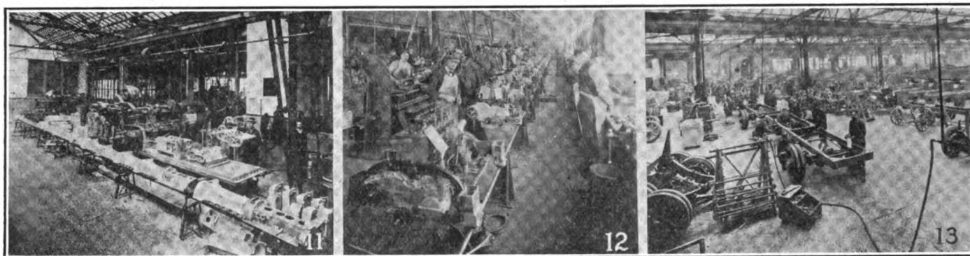
Key to illustrations of technical training in the truck department: 11, Machining operations on motor truck crank cases; 12, Motor adjustment on the conveyor where motors are assembled; 13, Where truck chassis are assembled and the practical points of truck chassis work are obtained
